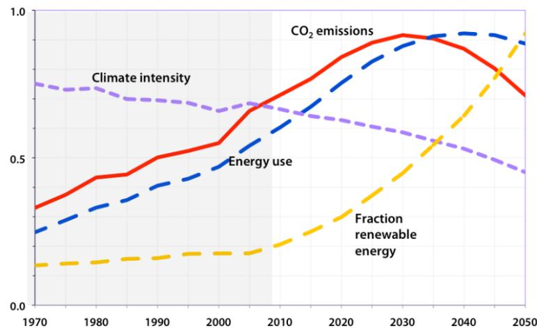
**Figure 10: World CO<sub>2</sub> emissions from energy use, 1970–2050.** Definition: Climate intensity = CO<sub>2</sub> emissions divided by total energy use. Scales: CO<sub>2</sub> emissions (0–45 billion tonnes of CO<sub>2</sub> per year); energy use (0–20 billion tonnes of oil equivalents per year); climate intensity (0–4 tonnes of CO<sub>2</sub> per tonne of oil equivalent); fraction renewable energy (0–40 per cent).
